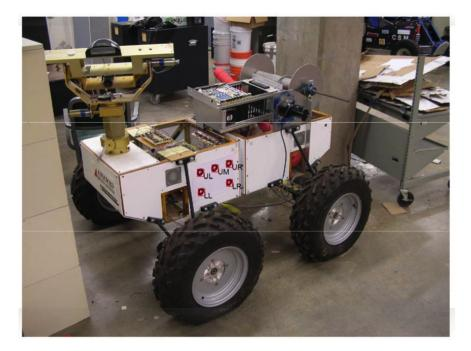
One approach is to look for features that are invariant with respect to pose. A simple invariant feature for this target is the co-linearity of the three top target circles. Regardless of pose, a set of three points that are collinear in 3D space will also be collinear in the image. So you could try all combinations of three detected features to find a set that is collinear. Identifying the order of the three features, and the two remaining features, is then pretty straightforward.
