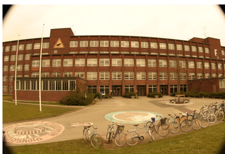
Figure 3: Radial distortion can not be handled with the K matrix. This requires a more complicated model.
