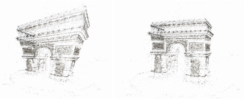
Figure 4: Reconstructions of the Arch of Triumph in Paris. Left: Projective reconstruction. Right: Euclidean reconstruction (known camera calibration). Both reconstructions provide the same projections.
