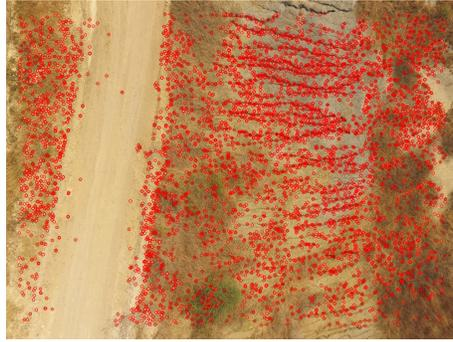
(a) Feature detection using HAHOG algorithm.
