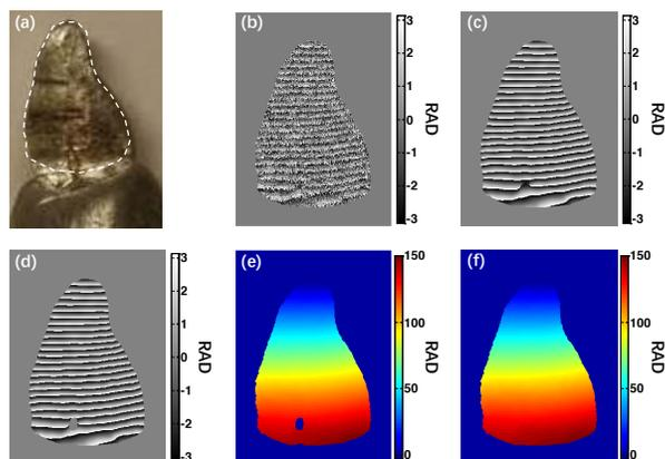
Fig. 2. Restoration of experimental phase data with WMPI, (a) tooth specimen, (b) wrapped phase with high noise and dislocation, (c) de-noised wrapped phase, (d) wrapped phase masked dislocation, (e) unwrapped phase and (f) final restored phase.
