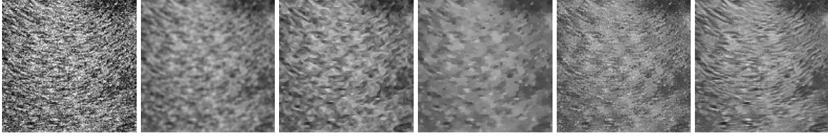
**Figure 3. Denoising experience on a natural texture. From left to right: noisy image (standard deviation 35), Gauss filtering, anisotropic filtering, Total variation, Neighborhood filtering and NL-means algorithm.**
